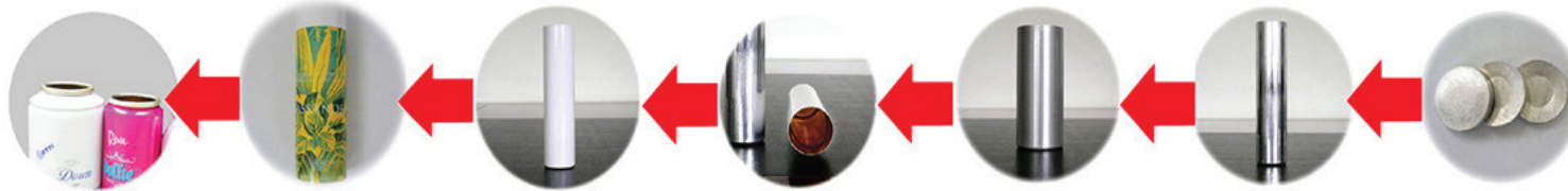
Necking machine Printing machine Base-coating machine Internal lacquering machine Washing machine Trimming machine Extrusion press machine
